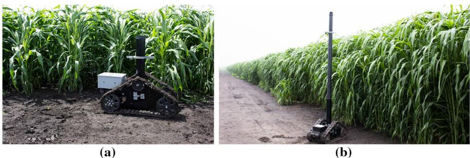
**Fig. 1** Photos of the TERRA-MEPP phenotyping platform operating in the field: **a** with a short mast configuration used for imaging plants early in the growing season, and **b** with the first version of a fully extended mast for measuring the height of tall sorghum
